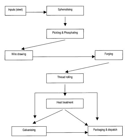
The Applicant provided the following diagram to illustrate the production process:
