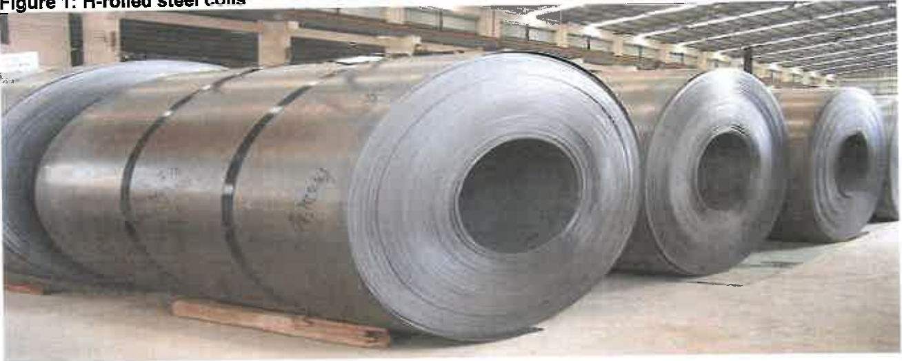
Figure 1: H-rolled steel coils
